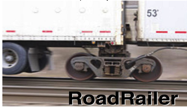
RoadRailer involves putting railroad wheels under trailers
