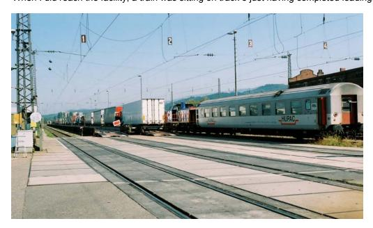
It consisted of 17 tractor-trailers on individual flatcars permanently affixed as a single platform, plus one passenger car, already occupied by the trucks' drivers. After a Swiss electric locomotive coupled on,
