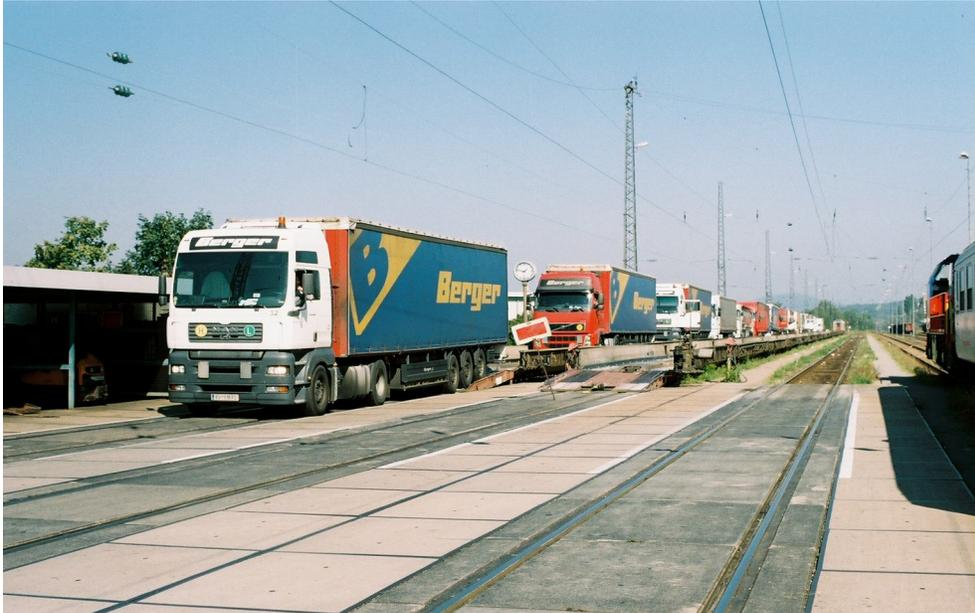
Trucks drive off a truck ferry train at Freiburg, Germany after an over-night rail journey from Italy. Truck ferry operations, widespread in Europe, help keep through trucks off the highways and reduce congestion, maintenance, and construction costs.
